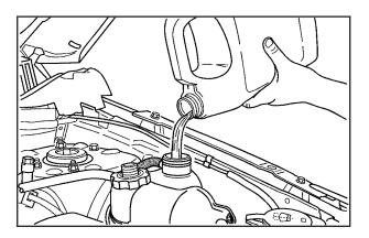
Fill the coolant surge tank with the proper DEX-COOL<sup>®</sup> coolant mixture, to the COLD FILL line.
